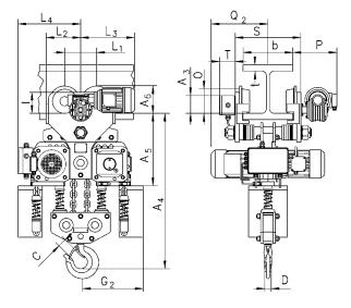
$\mbox{CPE}{\,}^1/\mbox{CPEF}$  with integrated electric trolley,  $10000\,\mbox{kg}$
