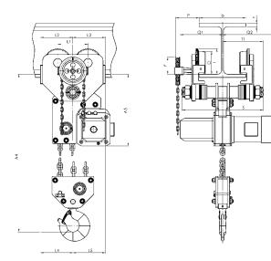
$\mbox{CPE}\,^{\rm 1}/\mbox{CPEF}$  with integrated geared or electric trolley, 7500 kg
