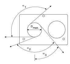
Rope lead-offs for electric winch RPE
