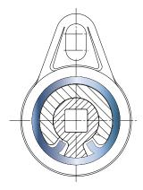
Brake new the spring has sufficient movement in both directions
