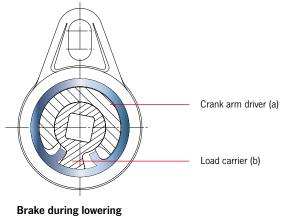
Spring (3) is released by the crank arm driver (a) and closed again by the load carrier (b)
