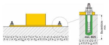
Standard base plate (welded) for anchor-bolt connection on existing concrete floor instead of welded-on base flange (only for operation inside a building) incl. HVZ dynamic anchor bolts.
