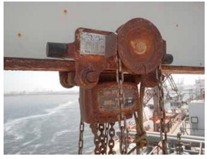
Corroded Yalelift with integrated trolley – still functional after 9 years in use
