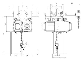
CPV/CPVF with integrated manual push or geared trolley
