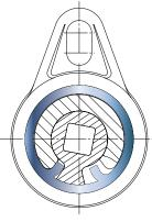
Brake, with braking torque applied during lifting
