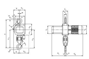
$\mbox{CPE}\,{}^1/\mbox{CPEF}$  with suspension hook, 3200 - 5000 kg, double fall
