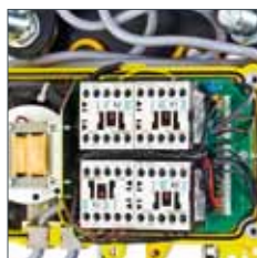
Increased operating safety through 42 V control voltage
