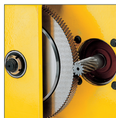
Gearbox with slip clutch
