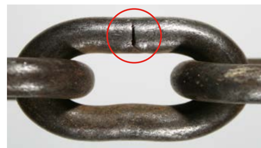
Clearly visible cracks
