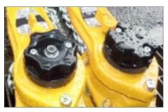
With the new design of the handwheel (on the right in the picture), the components of the brake remain unaffected by the incidence of humidity.
